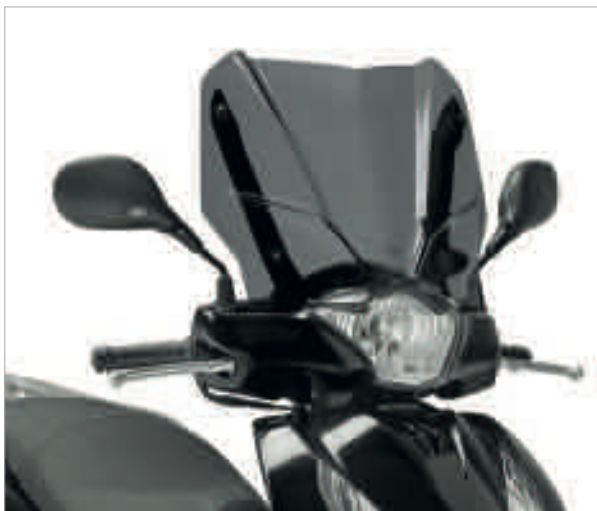
D1128S Honda SH 125i-150i (12 > 16) Specific screen smoked, to be fixed with original Honda fitting kit 36,5 x 45 cm (H x W)
