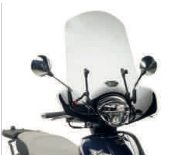
6109A+ A6109A Kymco Like 125-150 (17 > 18) Specific screen, transparent 49,5 x 65,5 cm (H x W) to be combined with the specific A6109A fitting kit
