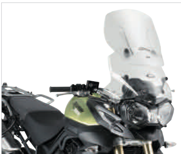
AF6401 Triumph Tiger 800 / Tiger 800 XC (11 > 17) Specific sliding wind-screen transparent, Airflow. Maximum height 60,5 cm (12 cm of extension) width 45,5 cm complete with specific fitting kit / to be mounted instead of the original screen
