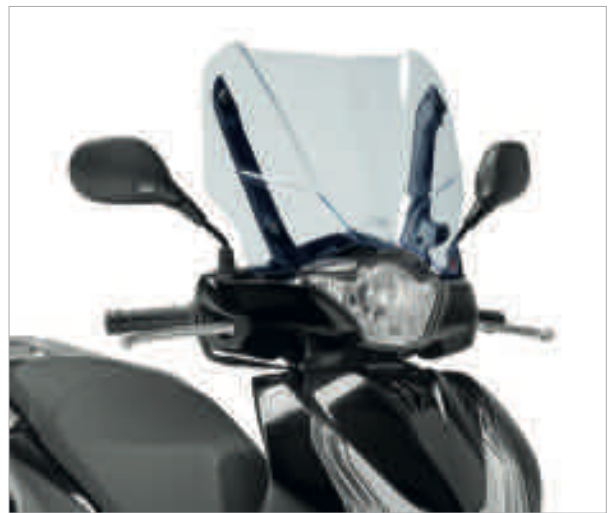
D1128BL Honda SH 125i-150i (12 > 16) Specific "ICE" screen to be fixed with original Honda fitting kit 36,5 x 45 cm (H x W)
